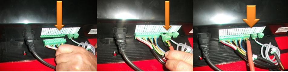
Turn on the control panel and make sure that everything has been connected correctly through activating automatic ignition function on the control panel.
