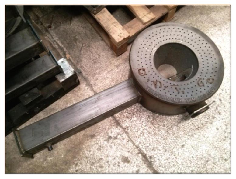
Cut in the hole in the oven and weld in metal nozzle performing the placement for the glow plug (ignition lamp)
