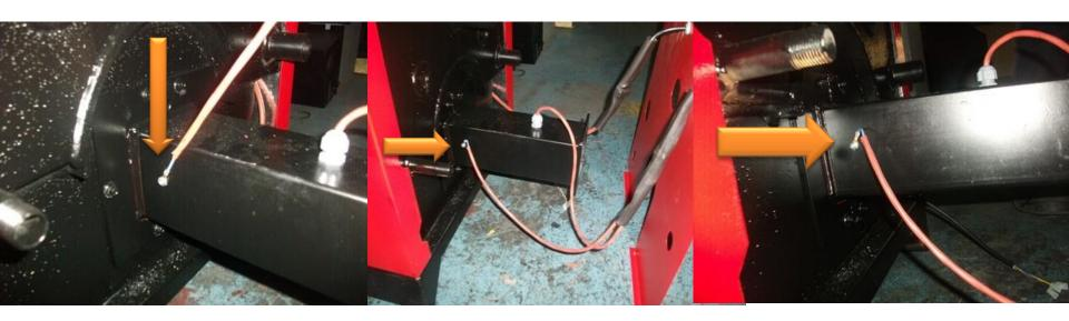
Pull the cable from the electrical power unit to the top cover metal sheet outlet and prepare to connect its socket to the control panel as shown below. Connect the socket to the control panel in respect with warning labels on the rear side of the control panel.
