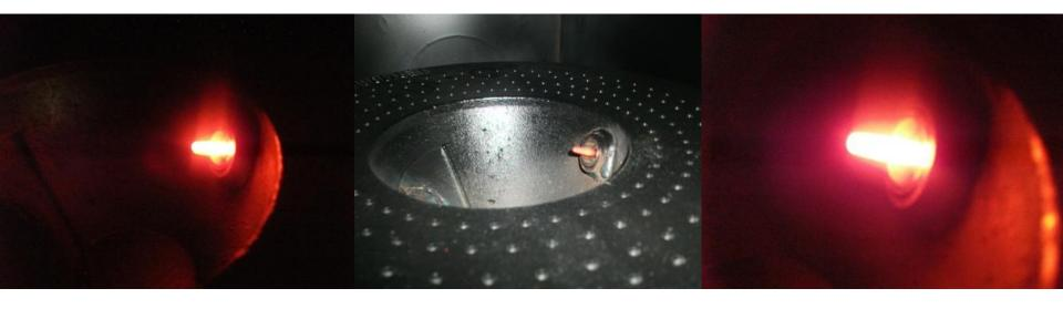
When automatic ignition is activated successfully, assemble the boiler with metal sheet covers.
