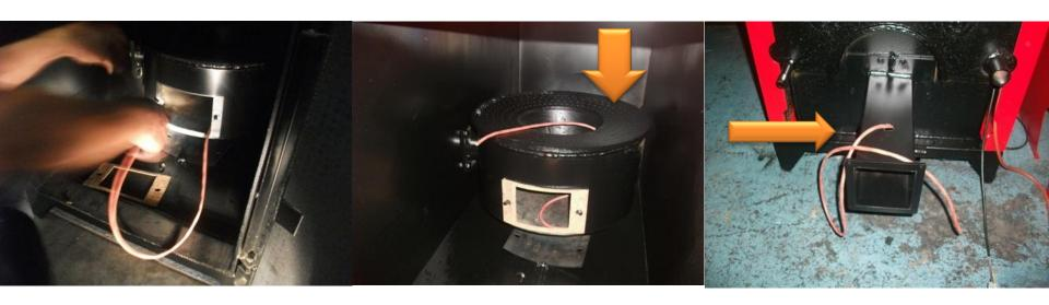
Prepare the wire coming out of the oven to fix the contactor for fastening the glow plug on following step. Fix the contactor as shown below.
