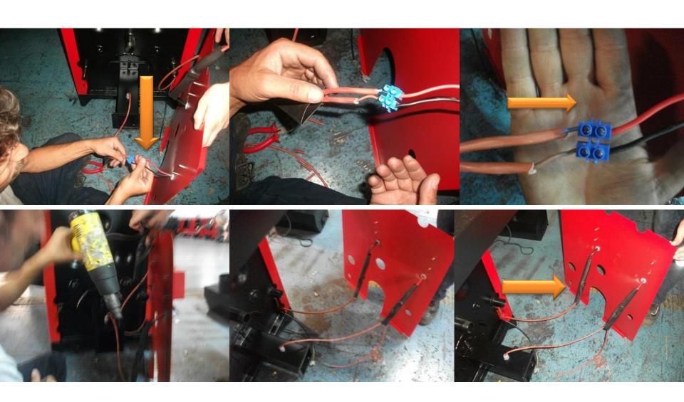
Screw in the bolt and connect the grounding cable.
