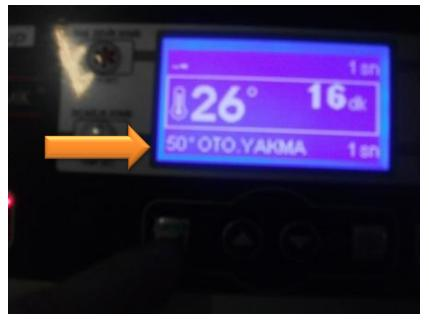
Make the initial trial ignition to be sure everything has been connected correctly and the automatic ignition is working properly. Follow the automatic ignition operating manual to execute this operation.
