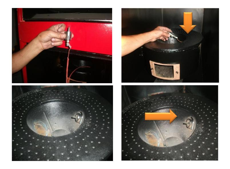
Fix tightly the cable coming our of the fan sleeve, prepare this cable to connect with the electrical power unit and afterwards connect it tightly to the socket coming out of the electronic power unit.
